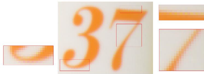
Figure 4. Result of the method that collects the pixels closest to the destination of the optical flow.
