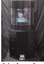
Figure 4 Cylindrical ray-based 3-D display
