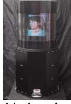
Figure 4 Cylindrical ray-based 3-D display
