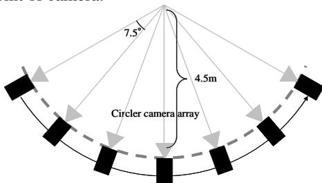
Figure 5 Camera array setup
