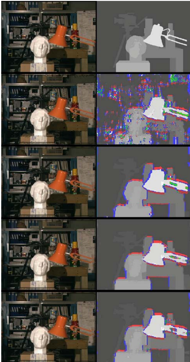
Figure 3. Free viewpoint images (left) and view dependent disparity map with occlusion map (right); From top to Bottom methods are GT, BM55, BP, MPDP, FMPDP. Blue regions are horizontal (left and right) occlusions and red regions are vertical (top and bottom) occlusions. Green regions are full occlusion regions.
